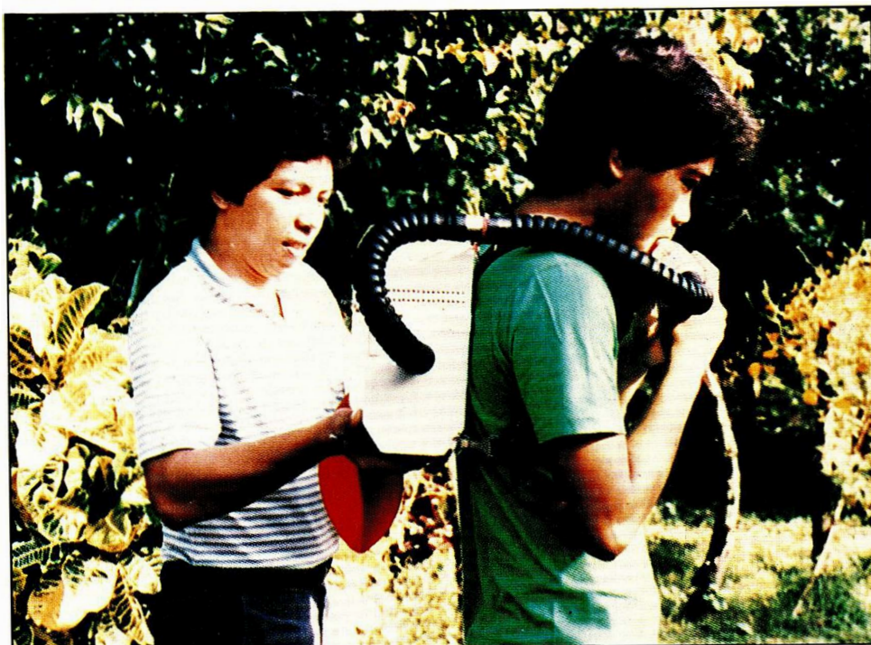
The Beckman E-2 oxygen analyzer is attached to measure energy expended while jogging.
